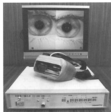
Fig. 1. Binocular electronic pupillometer (Newopto Corp. ET-200)
