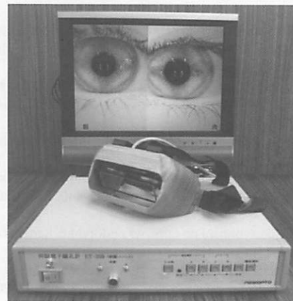
Fig. 1. Binocular electronic pupillometer
